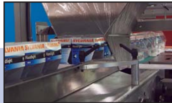
Plow Forms the Film Around the Package
