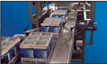
Flighted Infeed Conveyor Securely Transports the Product into the Sealing Area
