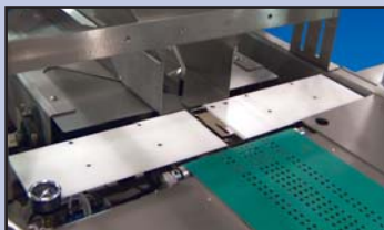
Bottom Seal Closes the Film from the Bottom
