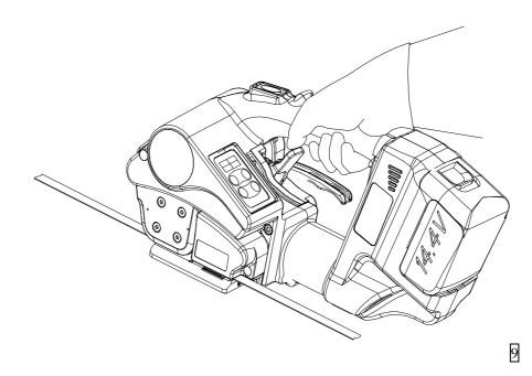
• Lift up the release lever and remove the tool (pict. 10).
