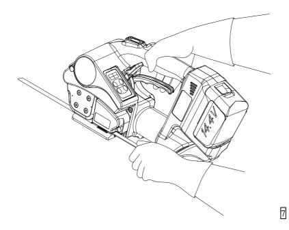
• Push the tension button until the programmed tension is reached (tension motor will stop) (pict . 8 ).
