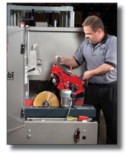
Combi's exclusive hinged case hold down plate allows for easy tapehead removal. Also, Combi's new open design eliminates overhead cross members in doorways, providing easy access for maintenance.
