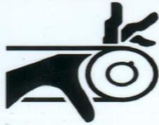
Moving parts can shear and cut.
