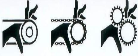
Moving machine parts can crush, cut and shear.
