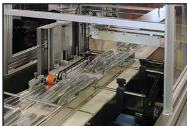
Horizontal Sealing System
