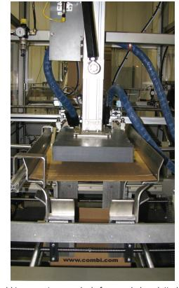
Combi tray erectors precisely form and glue slotted style trays, trays with tuck flaps and trays with one piece lids
