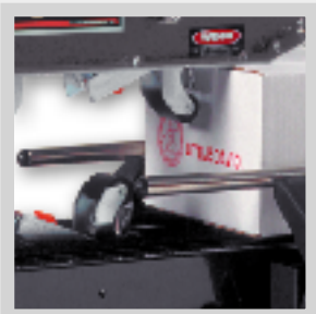
Self-centering side rails
