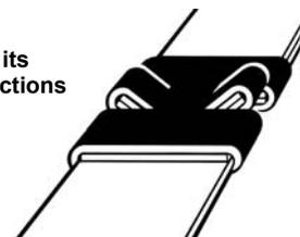
**NOTE: NOTCHES MUST BE EQUALLY SPACED ALONG THE ENTIRE LENGTH OF THE SEAL. FAILURE TO EQUALLY SPACE THE NOTCHES COULD RESULT IN STRAP SEPARATION. MORE THAN ONE SEAL MAY BE REQUIRED FOR CERTAIN APPLICATIONS - USE THE CORRECT NUMBER OF SEALS.**
