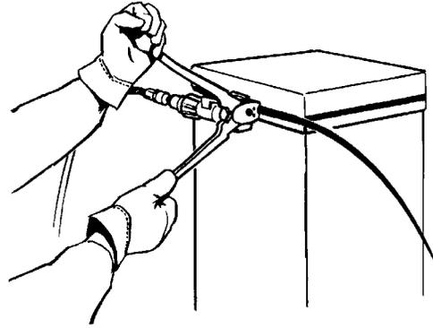
2. Bring the sealer handles completely together to assure a proper notch.
