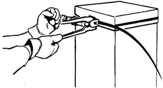
3. Remove the sealer and bend the loose strap sharply back on the seal. Several additional bends will result in a clean strap break-off. If the width and gauge of the strap being used will not allow it to be bent, cut the strap supply as close to the seal as possible using an approved strap cutter.
