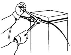
2. Bring the sealer handles completely together to assure a proper notch.
