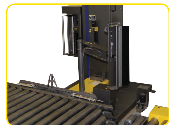
Film Clamp/Cut/Wipe Assembly Cuts and Attaches User-Friendly Operator Controls
