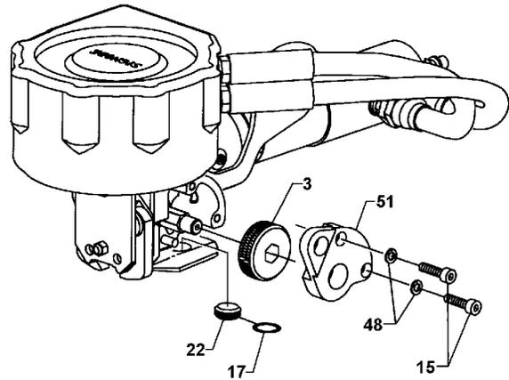
6. Check the feedwheel to wear pad clearance. The clearance between these parts should be .002" to .006" (0.05-0.15mm). Adjust the clearance as required by turning the M6 socket head set screw (Pg15, #14). Turning the adjustment screw clockwise increases the gap.
