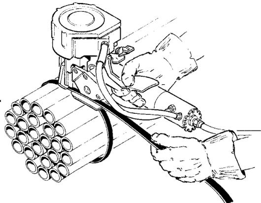
3. While continuing to hold the tool by the motor, release the stationary handle. Press the lever marked #1 to its locked position (tension) to begin tensioning the strap around the bundle. The tool will stall when the set tension level has been reached. If the tension is too much or too little, the tension can be adjusted as described elsewhere in this manual.
