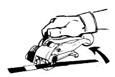
5. With left hand, pull top strap back and at an angle to the left, holding taut. Place base of tool just ahead of seal, cutter blade on the strap. Grasp knob of tensioning handle and slide tool forward to cut the strap. Inspect the joint to make sure it had been properly formed. Refer to the sealing tool manual for details regarding the joint.
