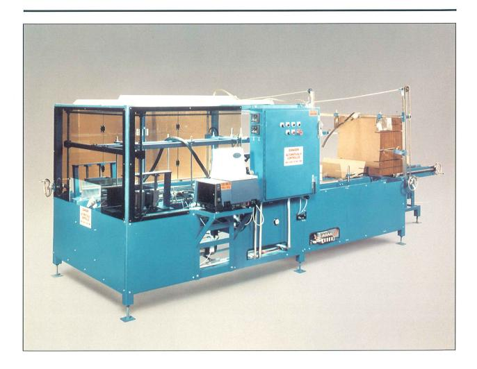
Will erect blank, accumulate product, load and seal tray or case blanks for a variety of canned or cartoned products. Converts in minutes to make complete wrap around type cases.
