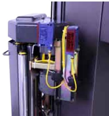
Kit includes second load height photo cell for additional turntable
