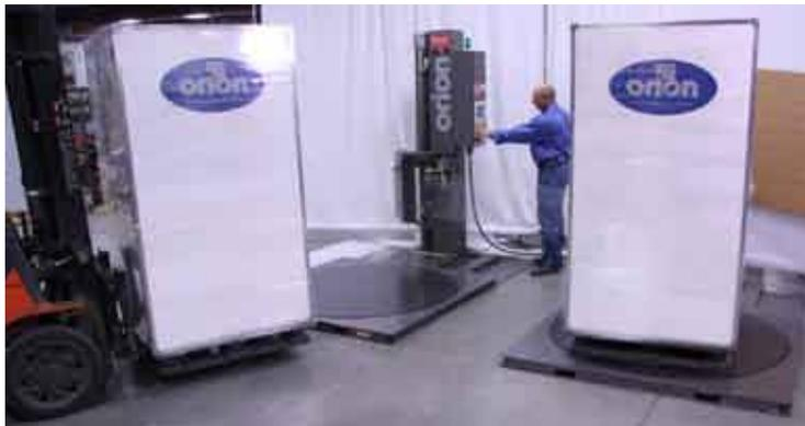
The carriage on the existing turntable easily reaches the second turntable.
