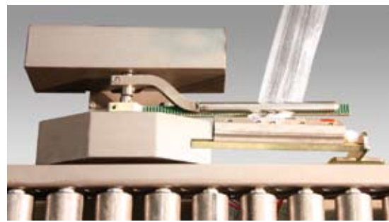
Pneumatically operated film clamp with high grip clamp for reliable grip & release of film tail
