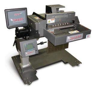
"Our all-in-one system evacuates air from the bag and allows the product to be gamma irradiated right in the bag." When the bag reaches the point of end use, its contents can be accessed by a transverse tear, similar to a cut made by a knife. This ease of opening, with no perforations required, reduces the chance of releasing package particles into the laboratory environment.
